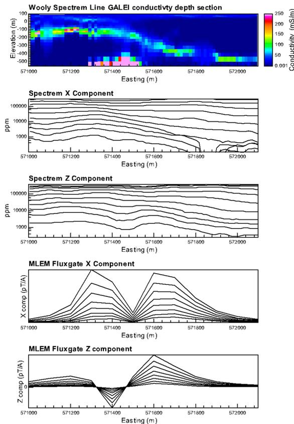
Figure 4. Spectrem GALEI conductivity depth section and line profile data over the Woolly target. The Spectrem data and inversion identifies a basement conductor. The ground MLEM clearly identifies an anomalous basement response.
