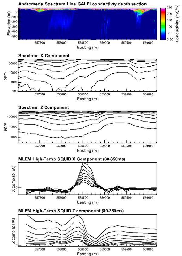
Figure 5. Spectrem GALEI conductivity depth section and line profile data over the Andromeda target. The Spectrem data fails to detect the basement response. The ground MLEM using a HT SQUID clearly identifies an anomalous basement response.
