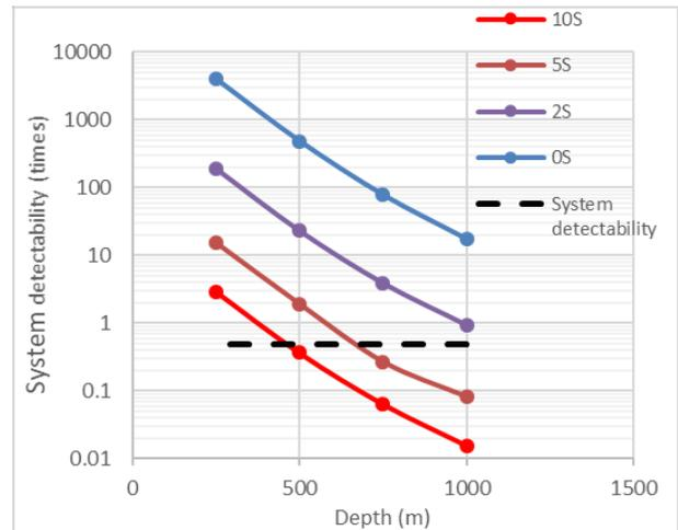
**Figure 2. System detectability of a 400 x 400 m 2,000 S flat lying conductive plate using a Low Temperature SQUID sensor in a slingram configuration with 400 x 400 m transmitter loop for various conductance overburden.**
